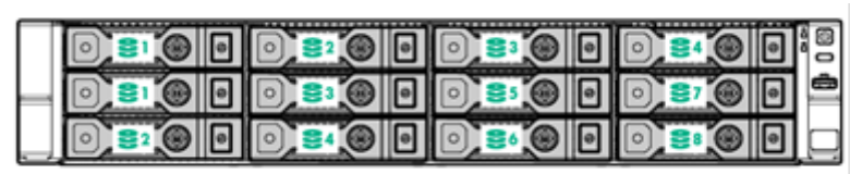
12-bay LFF hot-plug drive model
